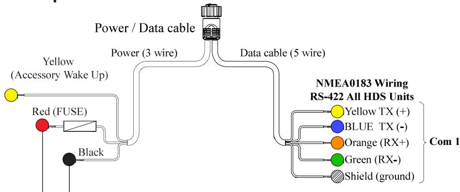
In this situation the Fishfinder/Chartplotter combo has a NMEA 0183 Yellow Tx(+) and Blue Tx(-). Both of these wires need to be used. The Yellow Tx(+) inserted to PIN 1 and Blue Tx(-) inserted to PIN 2, PIN 3 and PIN 4 are not used.
