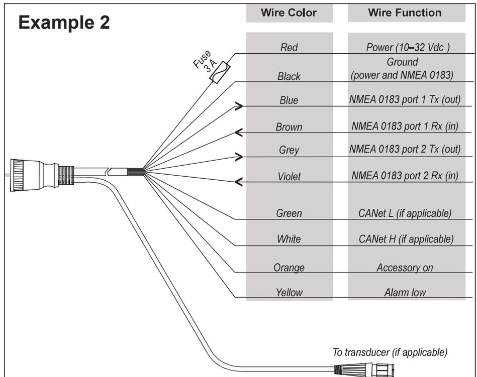
In this situation the chartplotter has two single-wire NMEA 0183 output wires that come out of their harness. The first is Blue, and labeled port 1 Tx(out), the second is Gray, and labeled port 2 TX-(out). If you are using port 1, the Blue wire should be inserted in to PIN 1; PIN 2 and PIN 4 should be linked together, and PIN 3 is not used. If using port 2 Gray wire, the above is the same but using Gray instead of Blue.
